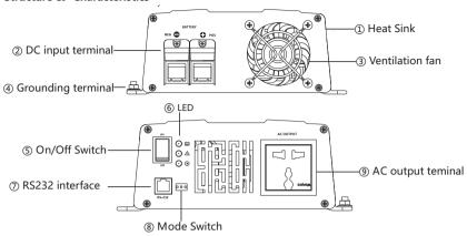
**Ventilation fan:** When the temperature of the radiator is greater than 40 ℃, the fan will be turned on; otherwise, the fan will be turned off.
